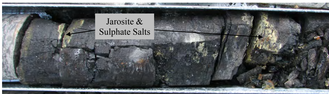
Plate 5: Jarosite and sulphate salts in coal from A Seam. Hole WAR2809, depth 153.7m.
