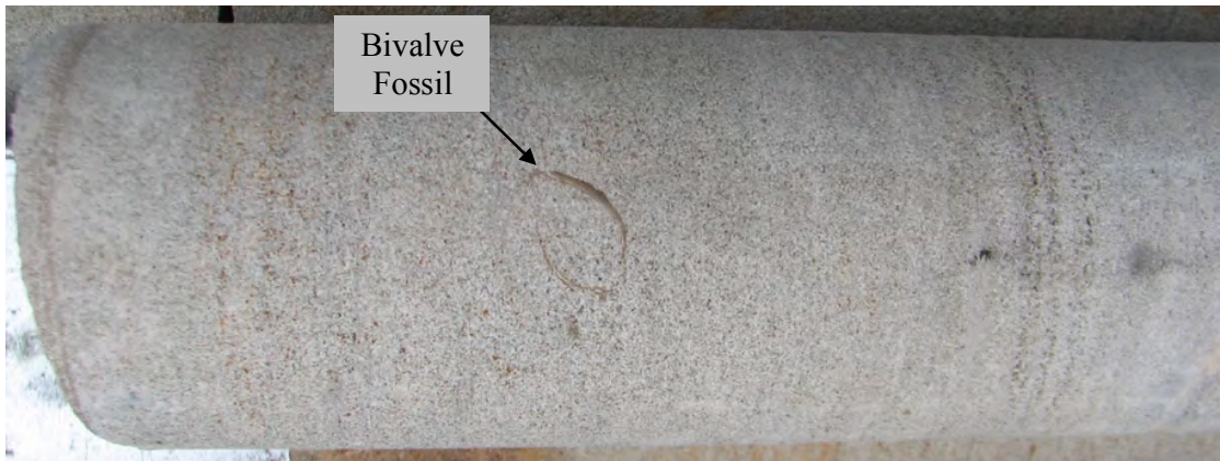
Plate 6: Sandstone with calcitic carbonate as grains or in the matrix, with bivalve fossil trace. Hole SK04, depth 70.7m.
