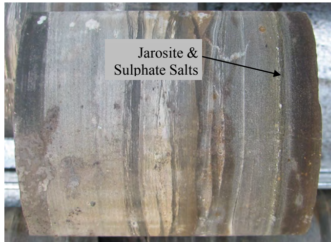
Plate 1: Jarosite and sulphate salts due to partial oxidation of pyrite associated with a thin carbonaceous layer. Hole SK04, depth 170.7m.
