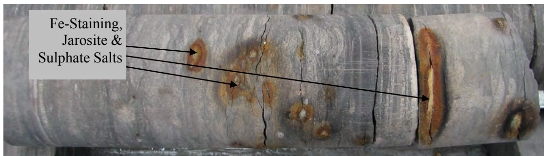
Plate 3: Iron staining, jarosite and sulphate salts due to partial oxidation of pyrite associated with carbonaceous layers and wisps. Hole WAR2809, depth 241.6m.
